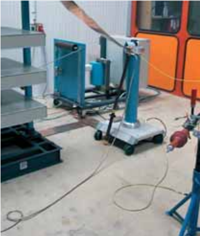
Equipment for impulse test up to 300 kV
