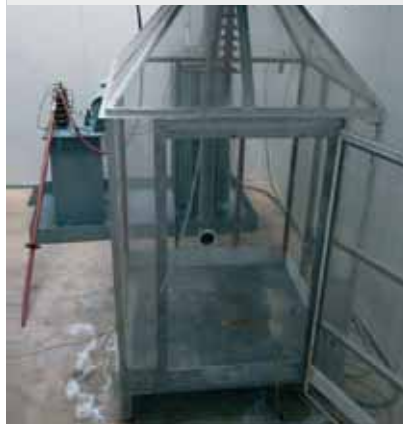
Saltfog chamber with AC transformer 50 kV
