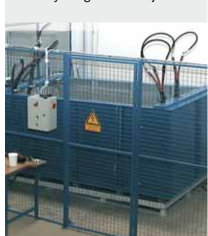
Water tank for submersed heat-cycling of cable joints
