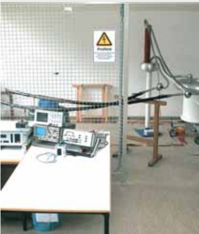
Equipment for partial discharge measurements
