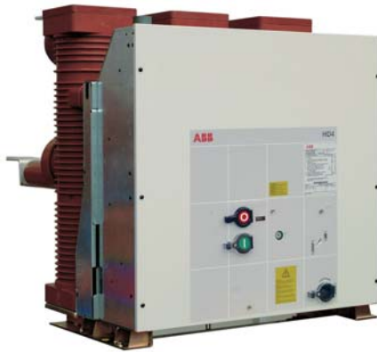
Fixed HD4 36 kV circuit-breaker with 275 mm pole centre distance: I_r = 1250-1600 A; I_{sc} = 25-31.5 kA; I_r = 2000-2500 A; I_{sc} = 20-25-31.5 kA.
